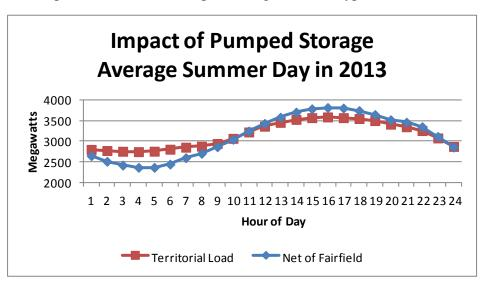
In effect the Fairfield Pumped Storage Plant was used to shave about 218 MWs from the daily peak times of 2:00pm through 6:00pm and to move about 2.4% of customer's daily energy needs off peak. Because of this valuable supply side capability, a similar capability on the demand side, such as a time of use rate, would be less valuable on SCE&G's system than on many other utility systems.
