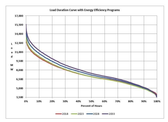
Figure C-2: Load Duration Curve with Energy Efficiency Programs and Before Demand Response Programs
