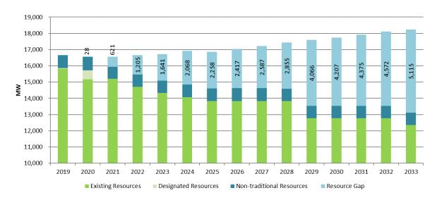
Figure 12-D: DEP Carbon Constrained Base Case Load Resource Balance (Winter)
