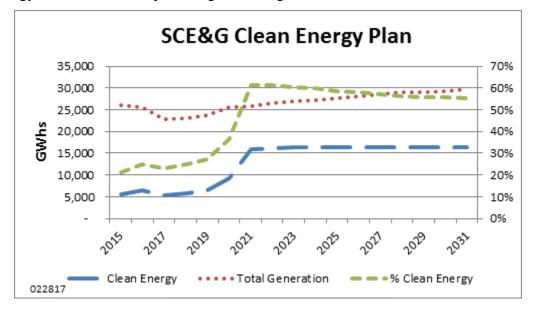
As seen in the chart above, SCE&G currently produces approximately 25% of its total generation from clean energy sources but by 2021 it expects to generate about 60% from clean energy. According to the EIA, the U.S. as a nation currently produces about 34% of its total generation
