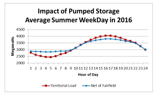
In effect, the Fairfield Pumped Storage Plant was used to shave about 307 MWs from the daily peak times of 2:00 p.m. through 6:00 p.m. and to move about 2.5% of customer's daily energy needs off peak. Because of this valuable supply side capability, a similar capability on the demand side, such as a time of use rate, would be less valuable on SCE&G's system than on many other utility systems.
