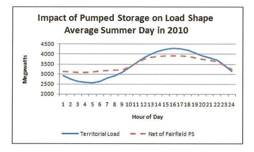
In effect the Fairfield Pumped Storage Plant shaved about 340MWs from the daily peak times of 2:00pm through 6:00pm and moved about 3.1% of customer's daily energy needs to the off peak. Because of this valuable supply side capability, a similar capability on the demand side, such as a time of use rate, would be less valuable on the SCE&G system than on many other utility systems.
