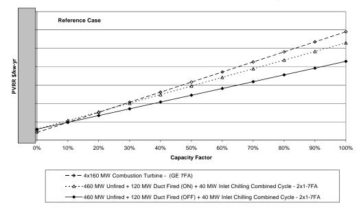
Note: The combined cycle alternative has been shown two ways in the above busbar chart: with the duct firing on and with it off. The unit alternatives are identical in that both curves include the capital costs of duct firing equipment; the only difference in the curves is the additional cost (loss in efficiency) to operate the duct firing equipment to achieve the higher level of unit capacity.
